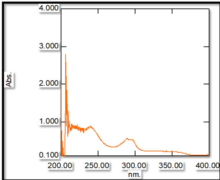
Fig. 2. Computerized display reading of absorption spectra of the extract taken from spectrophotometer
