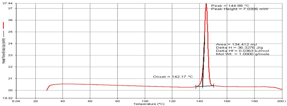
Figure 4: DSC Thermogram of pure clotrimazole
